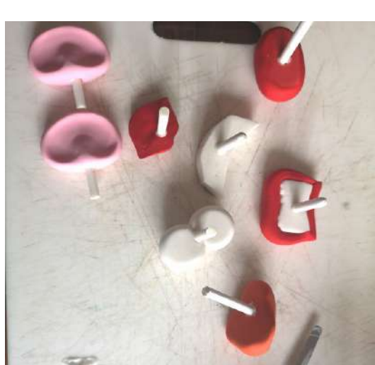
STEP 39 Using the glue, fill the hole in each accessory and insert the matching appropriately sized plastic dowel.
