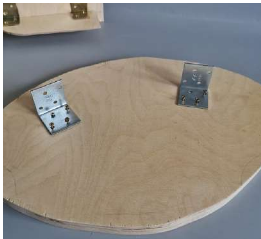
STEP 11 Attach the book to the cake board. Take 2 90-degree corner brackets and screw the bottom leg of each of them to the cake board at the correct angle matching the book.
