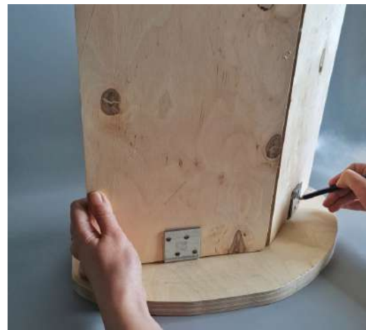
STEP 12 Position the base of the book to the screwed brackets and mark with a pencil where the brackets are attached on the back of the book cover.
