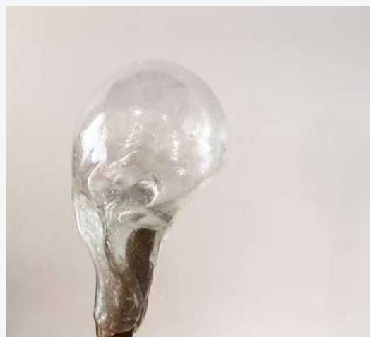
STEP 14 Start pumping air into the ball until you reach the size you want. Allow it to cool.
