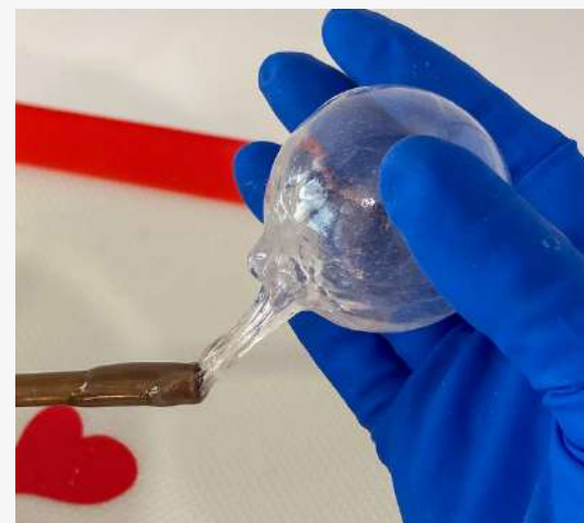
STEP 15 Heat the copper tube with the torch and with gentle semi-circular moves remove the ball.
