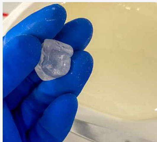
STEP 10 Transfer the isomalt to a silicone mould, let it cool down to a consistency that allows manual handling (when the isomalt doesn't stick to the gloves) and cut out a small ball with the scissors.
