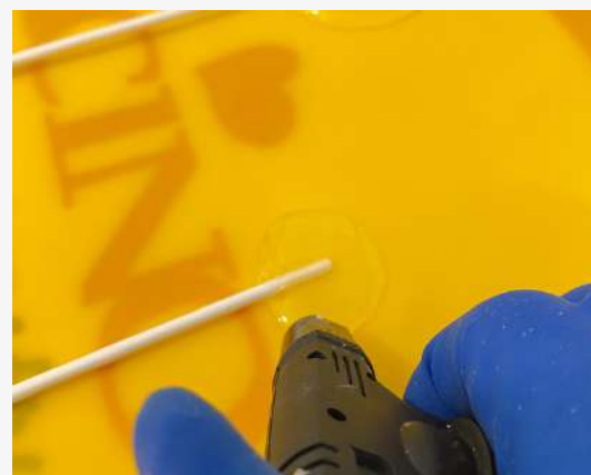
STEP 6 Use the heat torch to remove air bubbles and make the surface smoother and brighter.
