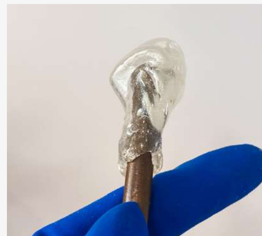
STEP 13 Adjust the isomalt closing it around the heated top of the tube.
