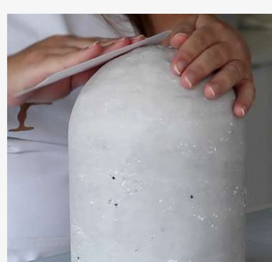
STEP 22 Smooth the joints using a flexible acetate smoother.
