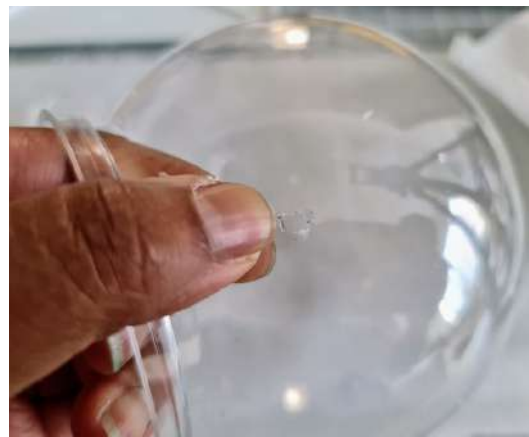
STEP 49 Using a knife cut a small hole in the bottom middle of the back of the dome, big enough to fit a drinking straw through, this is to allow you to make the snow move. Cut a similar sized hole 1cm above the first, this is to allow the air to expel.
