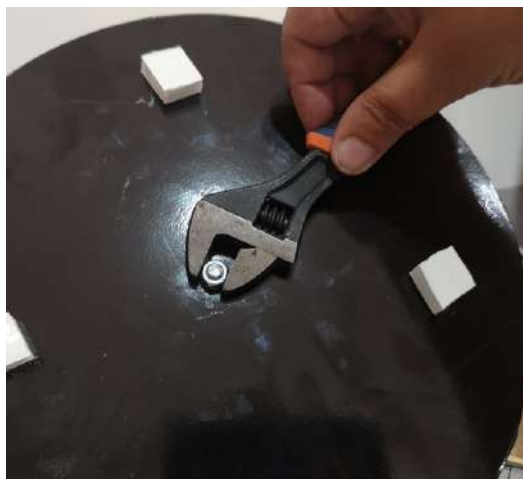
STEP 3 Assemble the structure as template 2. Always use a washer between the nut and the board. Screw the nuts tightly using a spanner.
