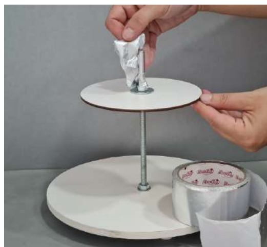
STEP 2 Assemble the structure as shown with nuts and washers both sides of each board - the upper board to support the head is to be approximately 17cm above the base. Cover the rod and fixings with stainless steel tape.
