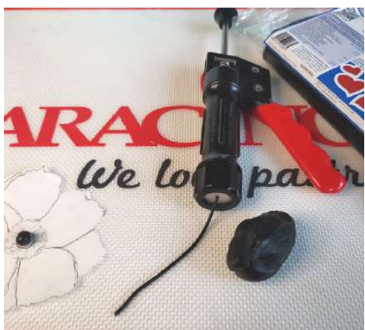
STEP 12 Using a 1mm hole in your extuder press long black strands. Roll a small ball for each centre of the flowers.
