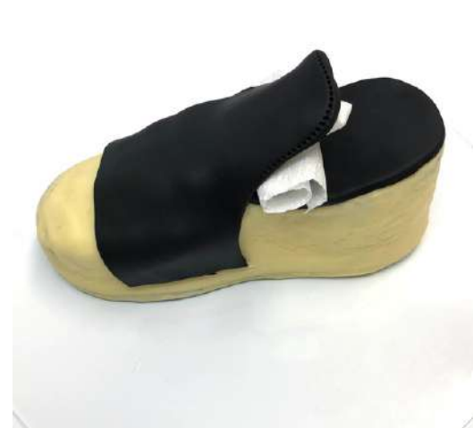
STEP 7 Cut out the tongue with the template and run a stitching wheel around the top section. Add this to your shoe and support until dry with rolled up kitchen paper.
