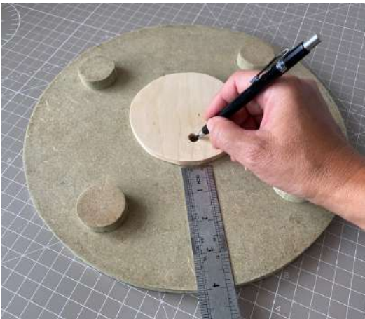
STEP 4 Prepare your cake boards. Drill a 8mm hole one inch away from the edge of the 4 inch cake board. Place the 4 inch board with the drilled hole 4 inches away from the edge of the 12 inch cake board as shown, this will be the front. Using a pencil mark the hole onto the board underneath. Drill an 8mm hole in your 12 inch cake board. Then hot glue some feet to the underside.
